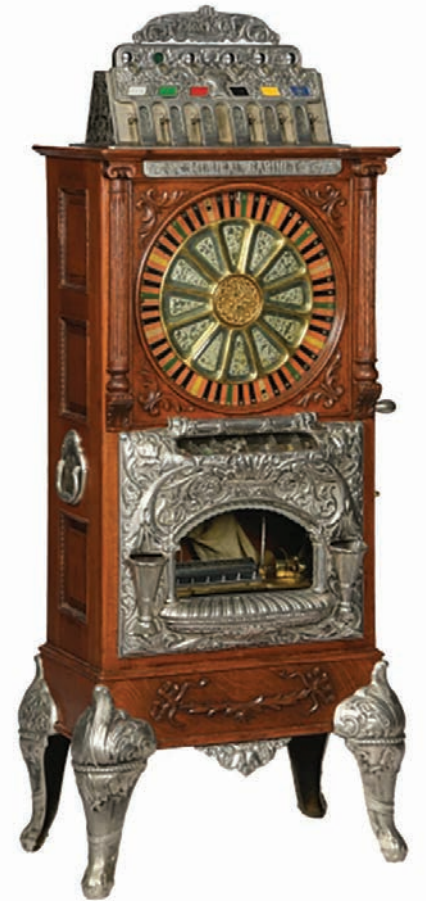
Above: Caille Bros. Manufacturing produced this 1904, 5-cent floor model slot machine housed in an oak cabinet. Players deposited nickels into their choice of seven-coin slots and pulled the level to spin the wheel and watch the ball bounce beneath the glass window. The color the ball lands on determines the payout. Estimate value of this machine is $180,000 to $250,000. (photo submitted)
