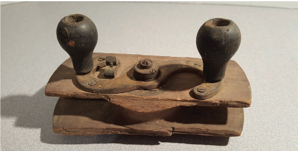
Above: Today’s electrician might look at this and discard it, thinking it’s worthless. Electricians of the past, though, would know it’s a reel for electric wire. The clip on top next the handle holds one of the wire. The user would then unspool the wire as they moved away to another location. This tool, from the mid-1800s, is valued at $400. (photo submitted)
