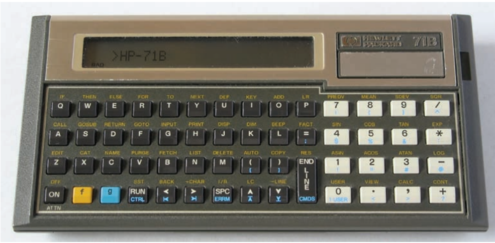
Above: The HP-71 series was fully programmable in the BASIC language. Notice keys labeled with commands like IF/THEN, FOR/NEXT, INPUT, and RUN which were fundamental instructions.
