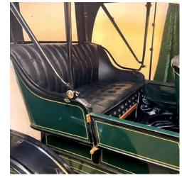
Above: The interior is in in good condition, as well as the cloth top which was replaced two years ago. A new wooden frame was put under the vehicle in 2009, as well as installation of a new 21-inch oversized boiler.
