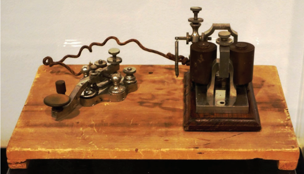
Above: On the left is a Western Electric Manufacturing Company key, circa 1876. The device on the right is a sounder that converts the signal into an audible sound. (Photo: Wikimedia Commons)
