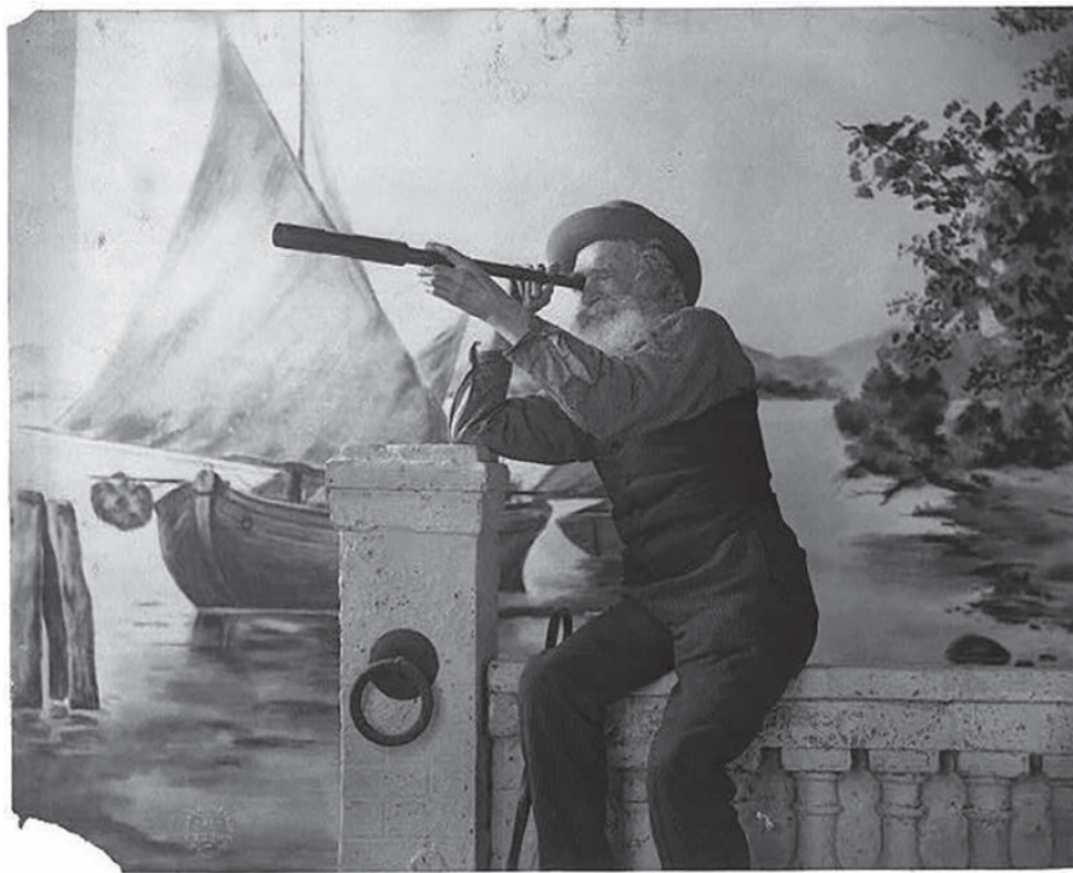
Above: A spyglass is a refracting variety that typically has extendable sections. They were used in nautical and military settings up through World War II.
