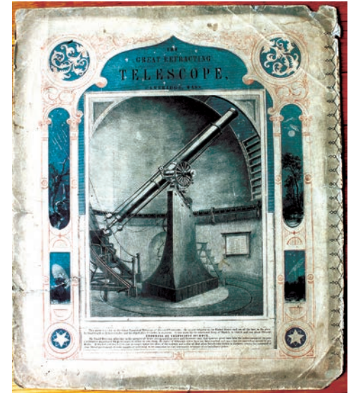
Above: Antique celestial illustration of the Great Equatorial Telescope at Harvard University in Cambridge, Mass., built in Munich in 1845-46, with a focal length of 22 feet 6 inches.
