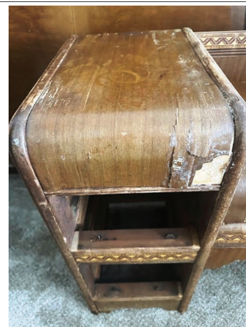
Above: This piece shows how badly damaged the veneer on waterfall pieces can deteriorate.
