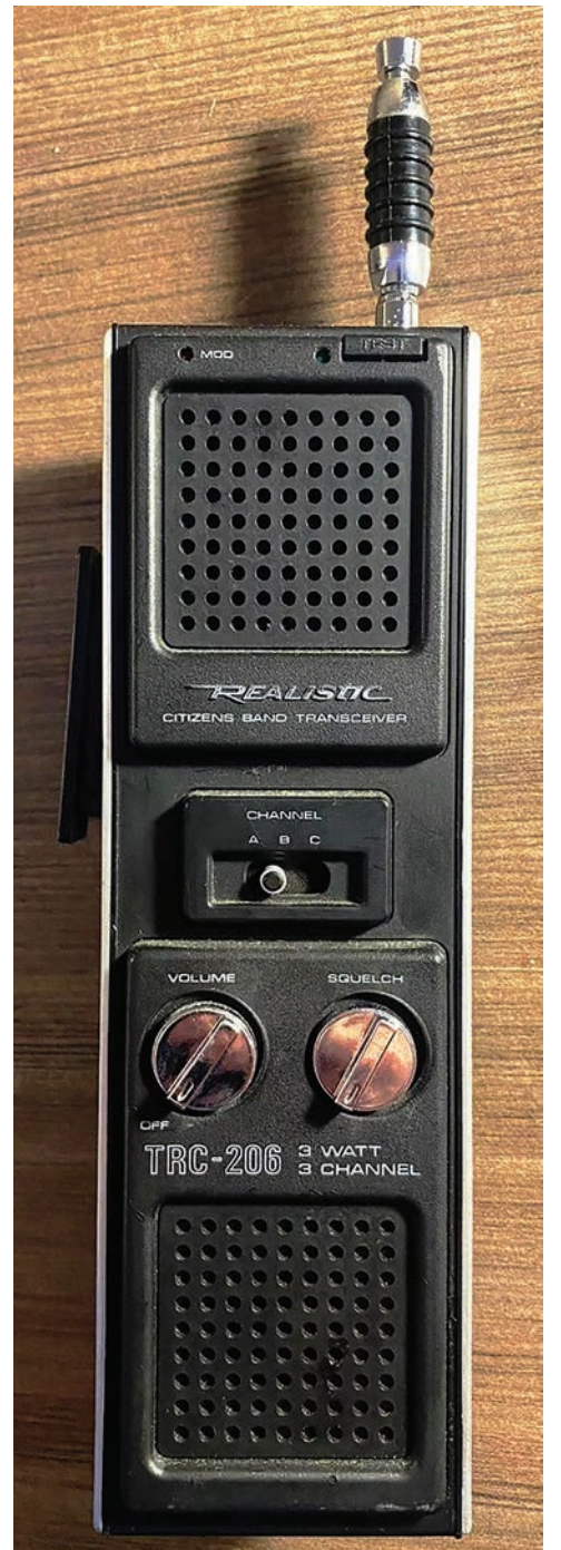
Above: This Realistic TRC-206 handheld had a full five watts of power but only 3 channels.
