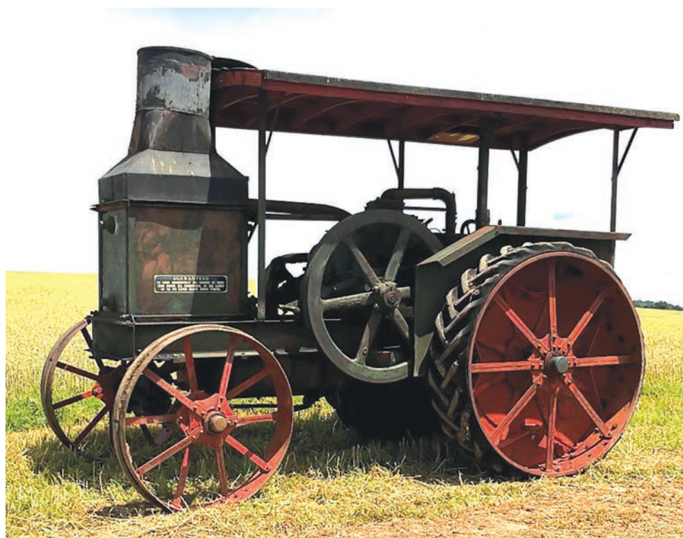
powered by a kerosene Higgins carburetor, delivering 16 HP on the drawbar
