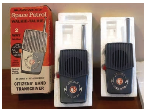
Above: Children's walkie-talkies of the era used channel 14 and had about 1/4-mile range.
