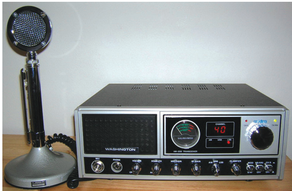
Below: The President Washington was a top-of-the-line base station, offering single-sideband and plenty of advanced features.
