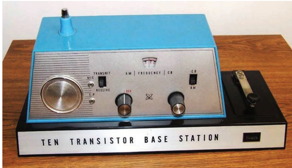
Above: This stylish unit was actually a low-power toy, operating on channel 14 to connect with other kids' walkie-talkies.
