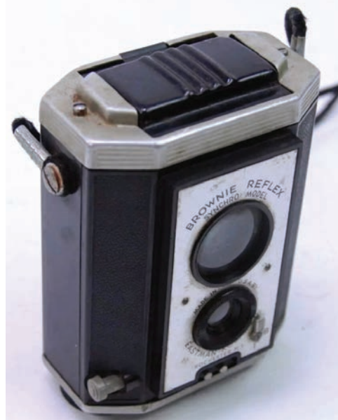
Above: Brownie Reflex models featured two lenses, one for taking the picture and one for reflecting the composition onto a screen at the top.
