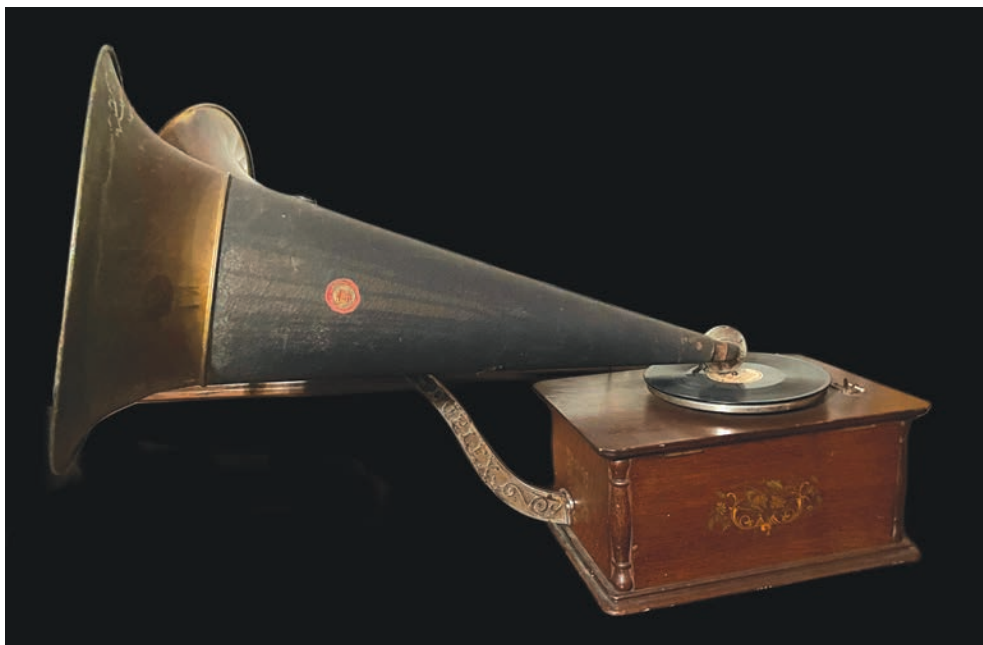
Above: A Kalamazoo Duplex phonograph. Available by mail order, this rare machine operated with a single reproducer using two horns.
