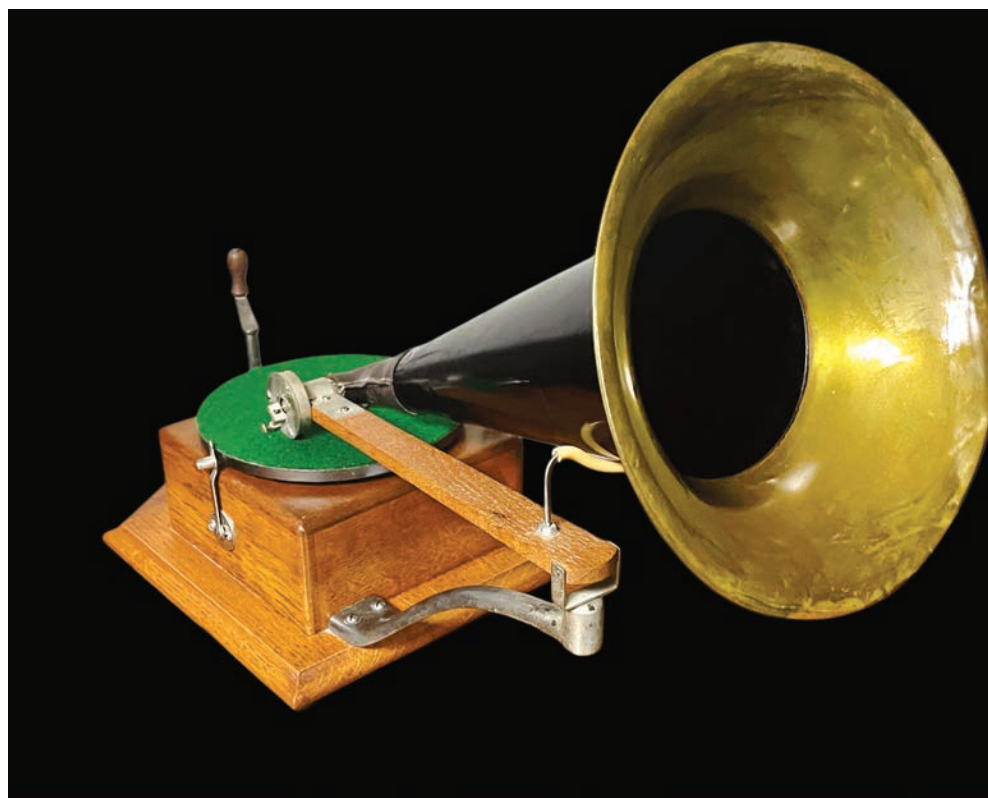
Below: An early Berliner phonograph. Emile Berliner transformed the recording industry with his use of flat discs instead of wax cylinders.
