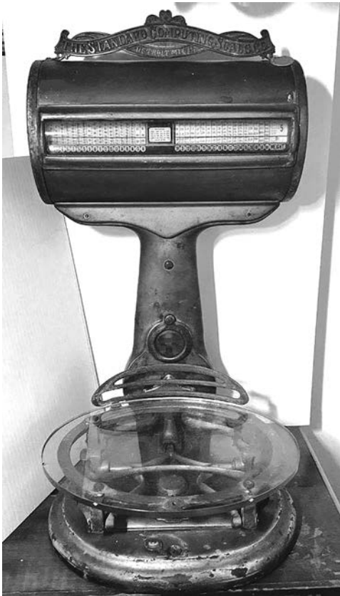
Above: Computing scales like this brass and cast-iron Detroit-made model ($72) could measure weight and compute costs.
